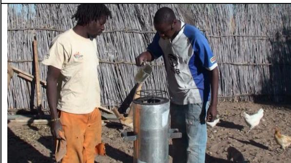
Water is poured onto the char after flames no longer come out of the top of the stove, to prevent the char from burning into ash.
