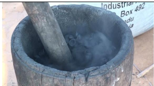
Charcoal from harder pieces of fuel, such as small pieces of wood, mangetti shells or maize cobs, needs to be crushed. If done immediately, then it will not be dusty as the char will still be wet from extinguishing.
