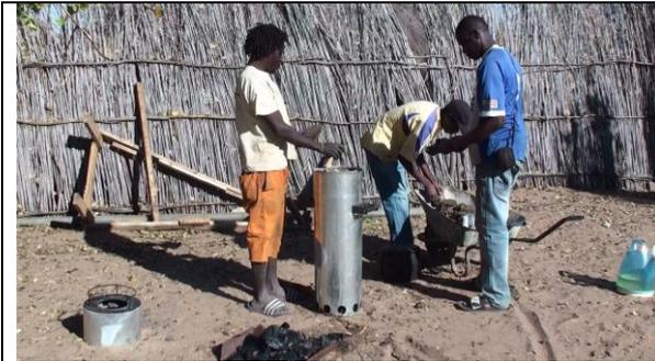
Small pieces of fuel are dropped into the stove. In this photo, the fuel is dry dung pats
